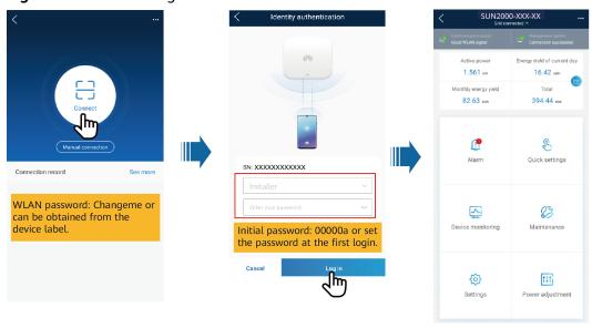
Figure 5-17 Connecting to the inverter
